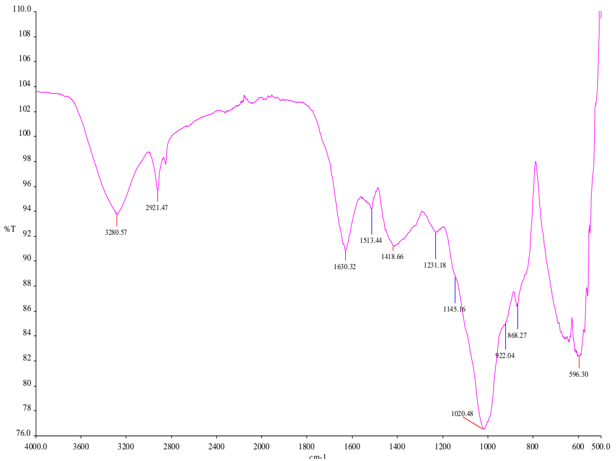
Graph-1b FTIR spectra of Neoscona theisi (Walckenaer, 1841) for without stretch silk fiber
